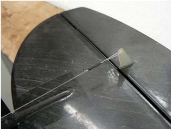
The rear end of the rudder cable in the working position.
