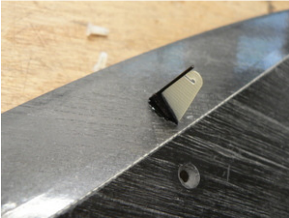
Elevator control horn installed with CA.
