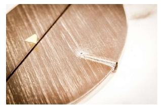
Make hole at the end of the boom support on the right side for right-handed launchers.
