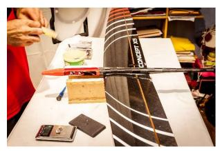
Use balance to get a good CG. With a long boom you normally need to insert some ballast on the nose.
