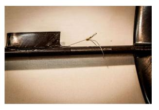
Continue the operation with this manoeuver. Create a loop on the boom. When you disassemble the elevator the wire stay still.
