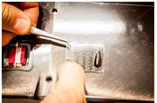
Install the aerodynamic cover with tape or use double-side tape.
