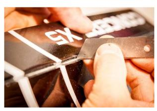
To turn the aileron easier use a cutter and pass the blade into the hinge.
