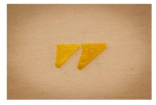
On the left is rudder horn, the other one is the elevator horn. Look at small difference of the two part. Use sandpaper for this horn to adujst it before applying CA.
