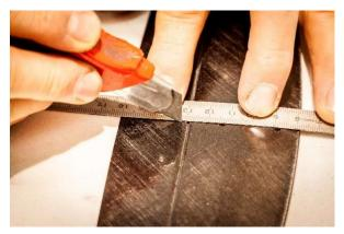
To install the elevator horn cut the elevator control surface on 12mm with a cutter aligned with the screw hole.
