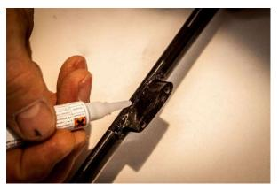
After this operation apply a fillet of CA or Epoxy on the support.
