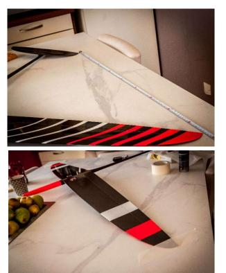
Before sticking the pod, please be careful about the symetry between the wing tip and the elevator tip. (LH and RH)
