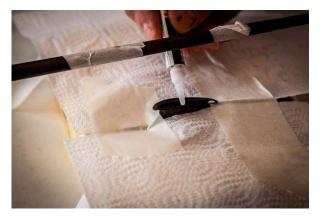
On this photo the stabilier is screwed onto the support
