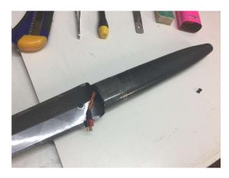
Use tool to drill hole for insert the wing wire
