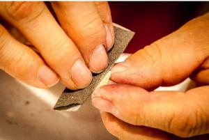
Before sticking the aileron horn, use sandpaper on the lower side.
