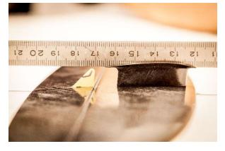
To check the size of the elevator horn, assembly the support and check with similar parts.
