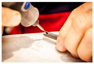
Now drill hole with tool on the rudder's support (Only to passed the rudder horn wire.)
