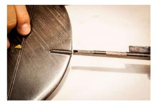
Now we are ready to apply a layer of Epoxy on the boom to stick the rudder.
