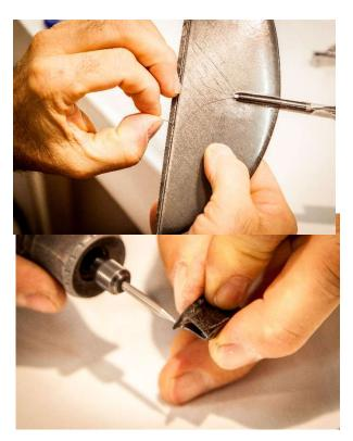
Insert the spring in the rudder, make a hole with the CAP and mark the position on the other side with a pen, install the second part.
