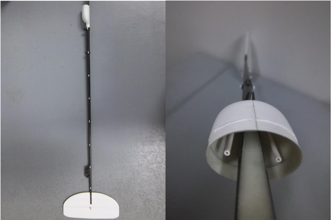
Picture 2.7. Pasting in the rod housing tubes
